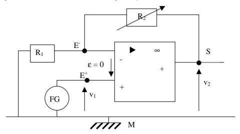
FG is a function generator giving input voltage v<sub>1</sub>.
