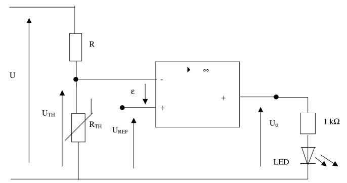
U = constant voltage = 10 V ;  $U_{REF}$  = reference voltage = 3 V;  $R_{TH}$  = resistance of a NTC type thermistor depending on temperature  $\theta$ . (The graph of  $R_{TH}$  against temperature  $\theta$  is given on page N°2) The operational amplifier is supposed to be ideal and functions **non-linearly**: Output voltage U<sub>o</sub> can take 2 values +V<sub>SAT</sub> = 15 V and - V<sub>SAT</sub> = -15 V.
