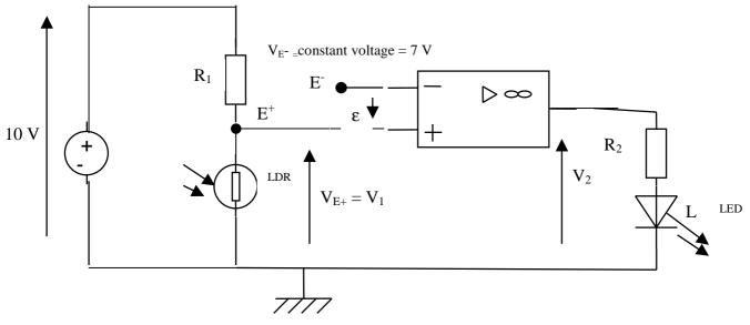
In presence of light the resistance of the LDR is equal to 1 k $\Omega$  and in absence of light the resistance of the LDR is equal to 10 M $\Omega$ .
