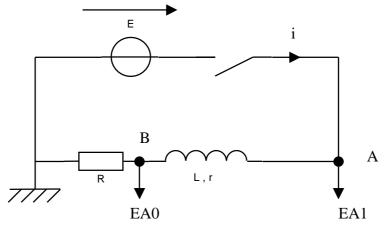
An electric circuit is composed of an ideal voltage source E = 10 V, a switch K , an inductor L with a resitance r ( real inductor) and a resistance R = 80  $\Omega$ .
