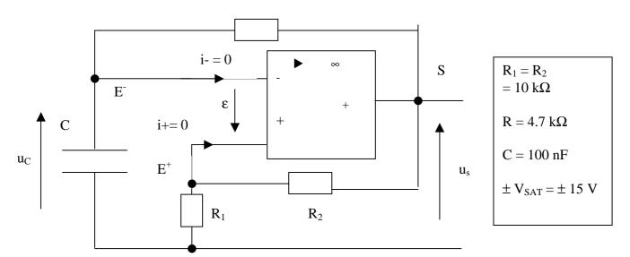
The <u>op amp</u> is supposed to be <u>ideal</u> and <u>functioning non-linearly</u>. Voltage  $u_S$  is a periodic signal of period T.
