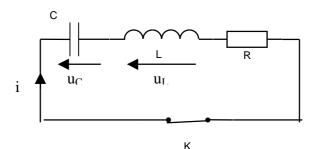
The capacitor C is initially charged at 4 V, L = 1 mH and the total resitance of the circuit is R
